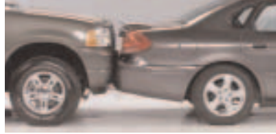
In a 10 mph front-into-rear crash test, damage was less (total $1,256) than to other pairs of vehicles in the same test.
