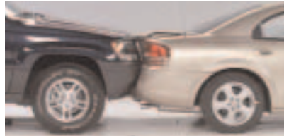
Bumper mismatch is the main reason damage repair costs exceeded $6,000 in the same 10 mph front-into-rear crash test.
