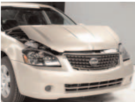
This Nissan Altima sustained a total of $4,507 damage when it struck the back of a Nissan Murano at 10 mph.
