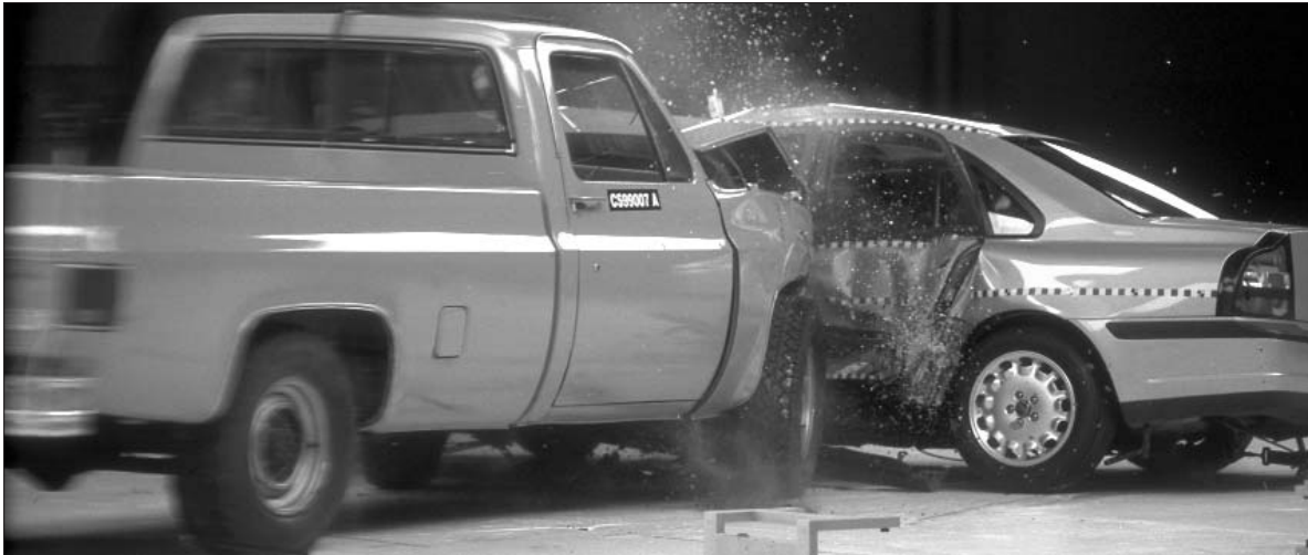
Crash test results: pickup (32 mph) into Volvo S80 (16 mph) with and without side airbag head protection
