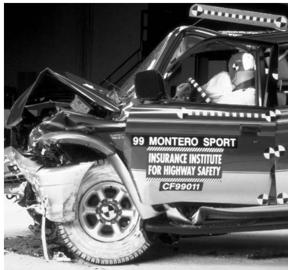
Mitsubishi Montero Sport rated poor
