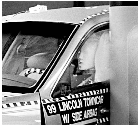
18 mph side-into-pole crash test: In a 1999 Lincoln Town Car with side airbag to protect the head and chest, the airbag kept the dummy's head from striking the pole
