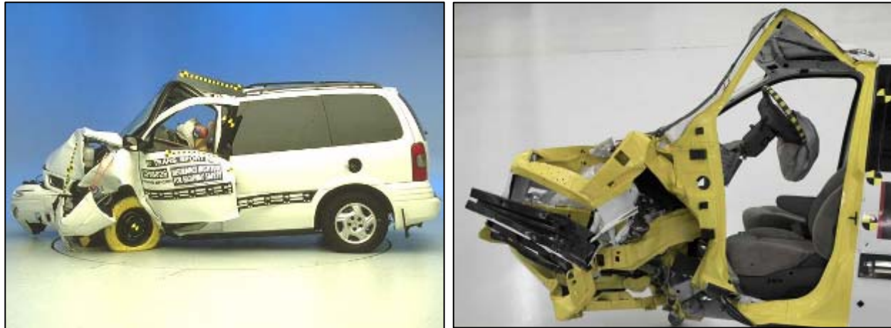
Figure 1 1997 Pontiac Trans Sport after Institute 64 km/h 40 Percent Frontal Offset Test
