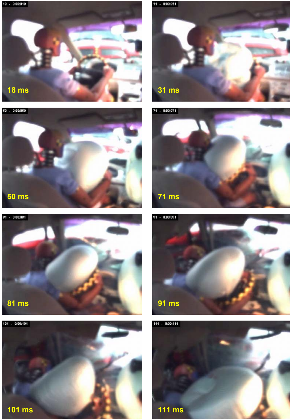
Figure 5 Onboard View of 1997 Honda Accord Driver Struck by 2002 Dodge Ram; Steering Column Moves Inboard, Preventing Airbag from Properly Cushioning Driver's Head
