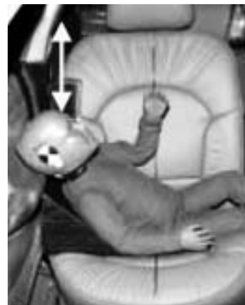
Auto manufacturers volunteered to conduct tests with dummies in positions where inflating side airbags might pose a hazard to children and out-of-position occupants in real-world crashes. Airbags that pass these tests don't pose any significant risks.
