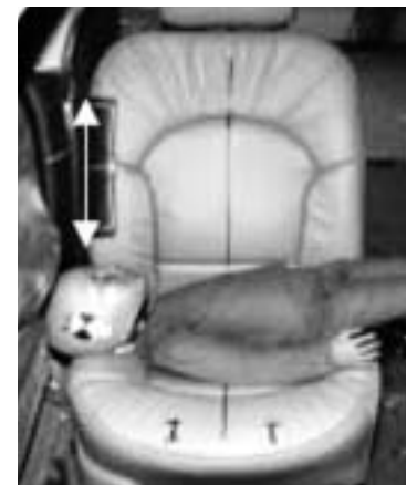
Auto manufacturers volunteered to conduct tests with dummies in positions where inflating side airbags might pose a hazard to children and out-of-position occupants in real-world crashes. Airbags that pass these tests don't pose any significant risks.
