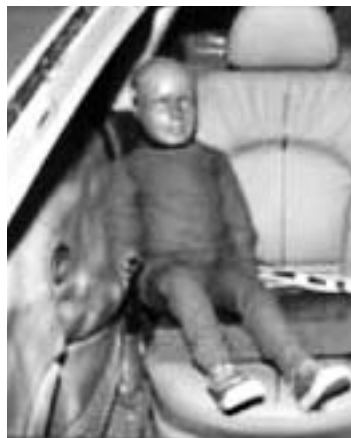
Auto manufacturers volunteered to conduct tests with dummies in positions where inflating side airbags might pose a hazard to children and out-of-position occupants in real-world crashes. Airbags that pass these tests don't pose any significant risks.
