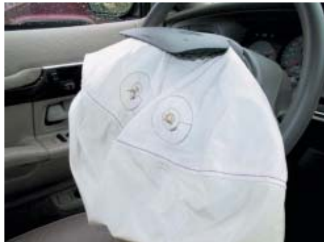
The driver airbags in these 1998 and 1999 models with depowered airbags offered equivalent or improved occupant protection, compared with 1997 models manufactured before NHTSA changed the rules to allow depowering.
