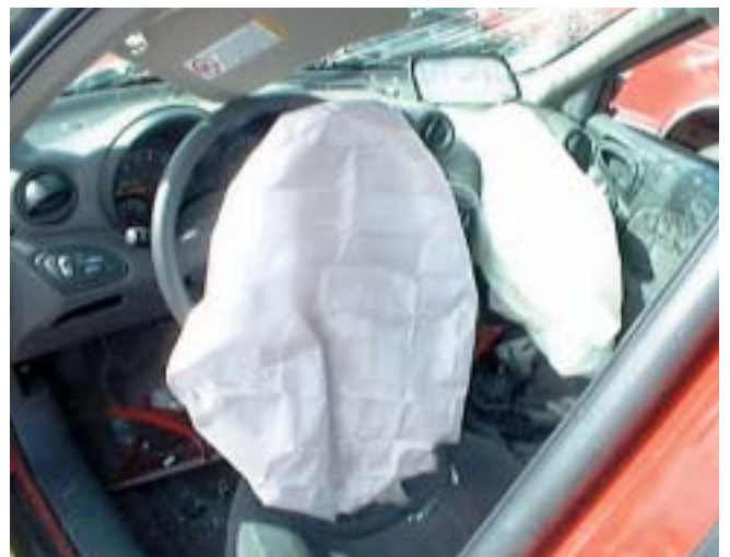
The driver airbags in these 1998 and 1999 models with depowered airbags offered equivalent or improved occupant protection, compared with 1997 models manufactured before NHTSA changed the rules to allow depowering.
