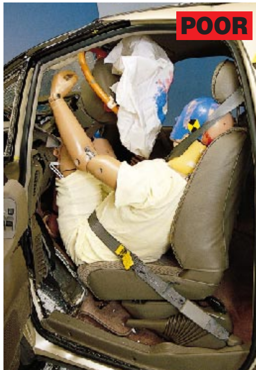
Dummy movement in the frontal offset test of the 1995 Passat (top left) wasn't well controlled so the dummy's head finished between the roof rail and the door frame. This problem has been fixed in the 1998 model (top right). There was significant occupant compartment intrusion in the test of the 1996 Previa (bottom left), the Sienna's predecessor. Too much belt slack allowed the dummy to submarine under the belt. The 1998 Sienna (bottom right) held up well — especially the driver space — in the offset test.
