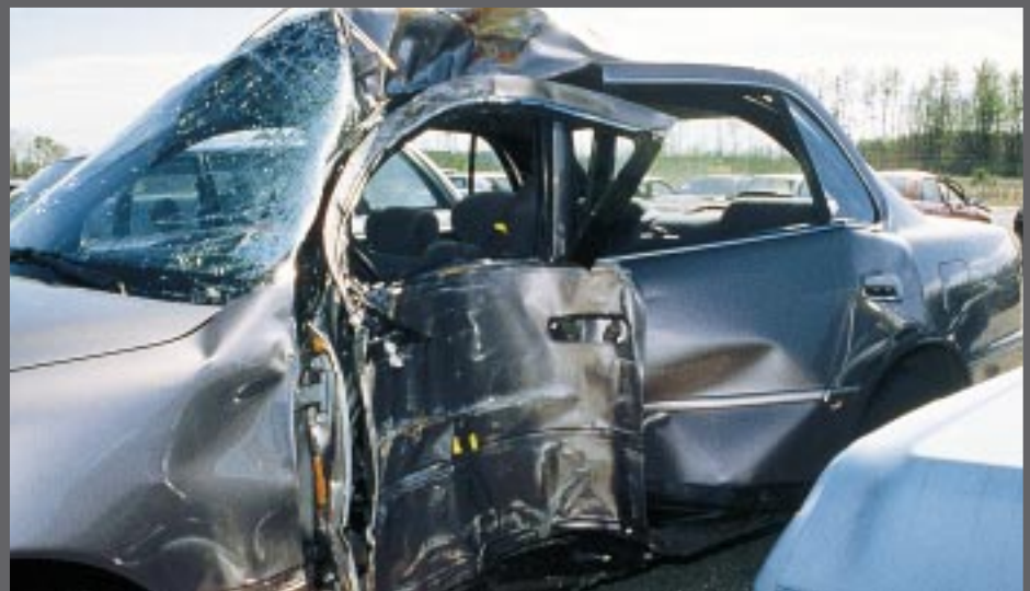
A 1993 Toyota Camry left the pavement during a left turn at an urban intersection. It hit a utility pole, spun out, hit a switch box, and then hit the pole's guide wire.
